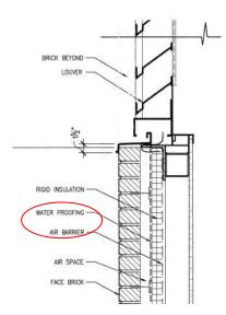
Figure 5. Exterior Wall Section indicating Weather-Proofing
