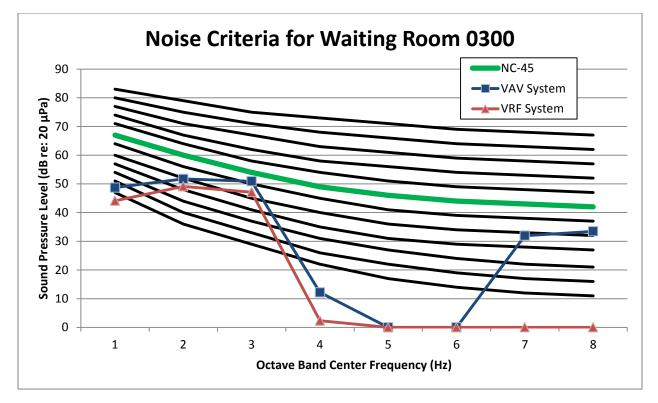
Figure 20. Noise Criteria Curve
