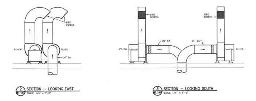
Figure 3. Bird Screens and Goosenecks
